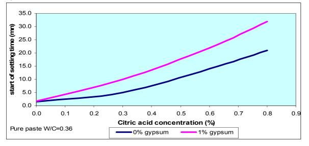
Figure 4: ADJUSTMENT OF PNC SETTING TIME
