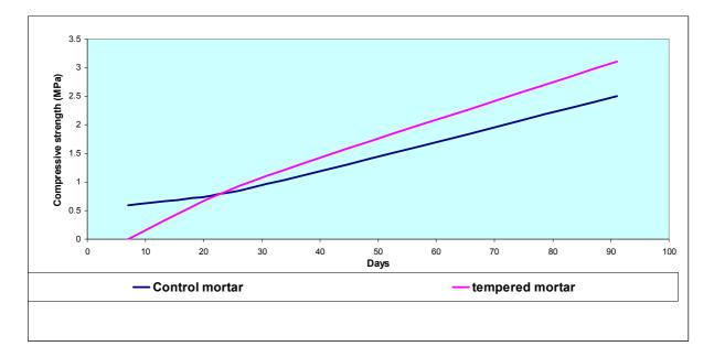
Figure 18: RISE IN STRENGTH OF A TEMPERED MORTAR
