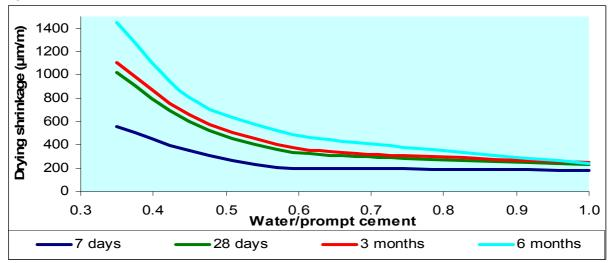
Figure 7: SHRINKAGE VS. W/C RATIO
