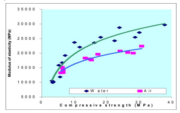
Figure 9: ELASTICITY MODULUS VS. COMPRESSIVE STRENGTH
